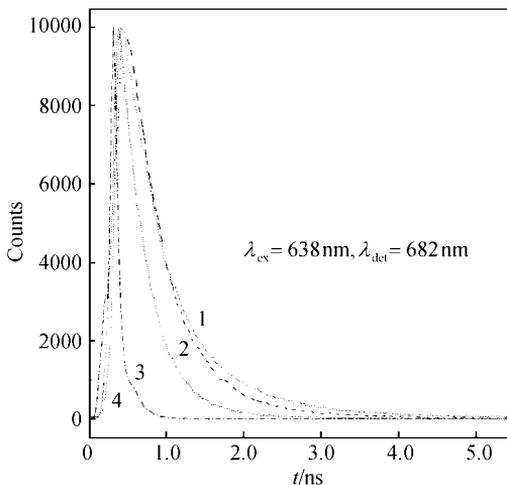
Fig. 4. Instrument response curve and fluorescence decay curves in PS II at room temperature for 1, water hyacinth; 2, spinach; 3, pseudo ginseng; and 4, laser.
