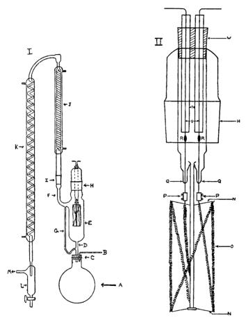
Condensers J and K may be of any efficient type. In the apparatus illustrated J is a double spiral condenser 50 cm. long, and K is a single spiral 90 cm. in length. The two are connected at the tops by a glass seal. The liquid trap L sealed to the lower end of condenser K is constructed of 35 mm. tubing and is 125 mm. long, with a stopcock for removal of liquid from the trap. The ketene or butadiene is conducted away through the tube M, of 8 mm. diameter.
