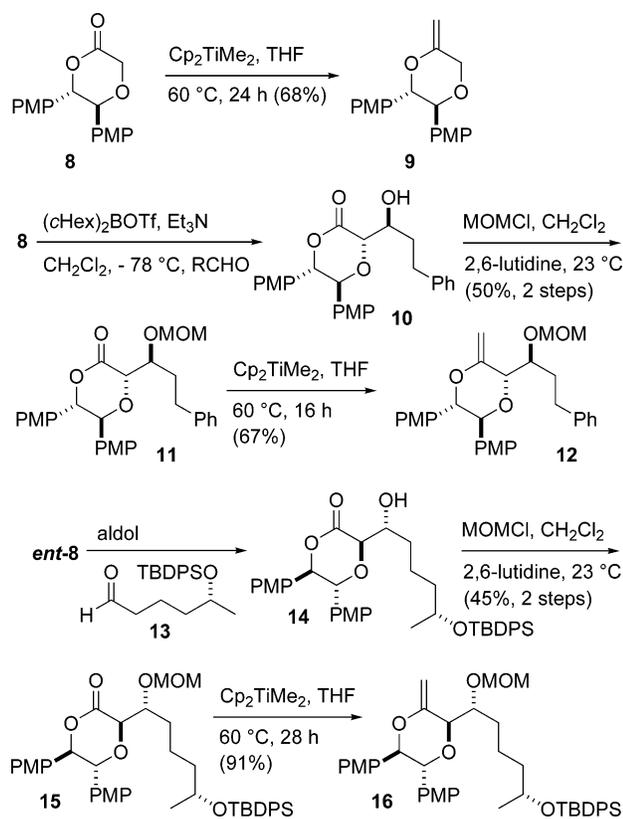
used immediately after the olefination reaction. The other compounds (**12** and **16**) could be purified by chromatography on aluminum oxide. The results of our study with lactone **8** and derived enol ethers are collected in Table 1. Compound **11** was obtained by *anti*-aldol reaction of **8** with phenylpro-
