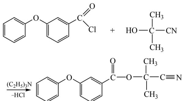
The synthesis was performed at room temperature (20–25°C) under stirring for 1 h using the 3-phenoxybenzoic acid chloride–acetone cyanohydrine–triethylamine in a molar ratio 1:1.2:1.2.
