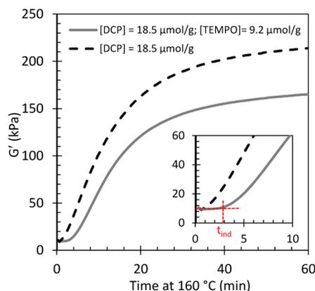
**Figure 2.** Dynamics of DCP-initiated LLDPE cross-linking. Inset: expansion illustrating reaction induction time.
