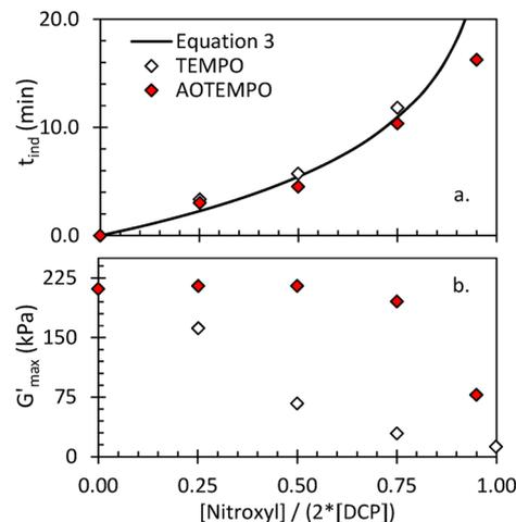
**Figure 4.** Influence of TEMPO and AOTEMPO on DCP-initiated LLDPE cure dynamics and yields ( $[\text{DCP}] = 18.5 \mu\text{mol/g}$ , 160 °C).
