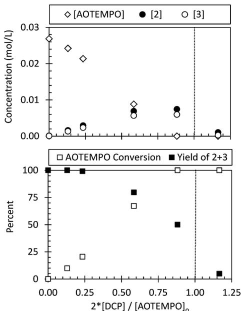
**Figure 1.** Model compound reaction products as a function of DCP loading: (top) reagent and product concentrations; (bottom) AOTEMPO conversion and alkoxyamine yields ( $[AOTEMPO]_0 = 0.027$  mol/L;  $160$  °C).
