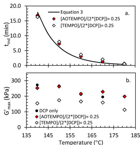
**Figure 6.** Influence of TEMPO and AOTEMPO on DCP-initiated LLDPE cross-linking induction times and yields ( $[\text{DCP}] = 18.5 \mu\text{mol/g}$ ).
