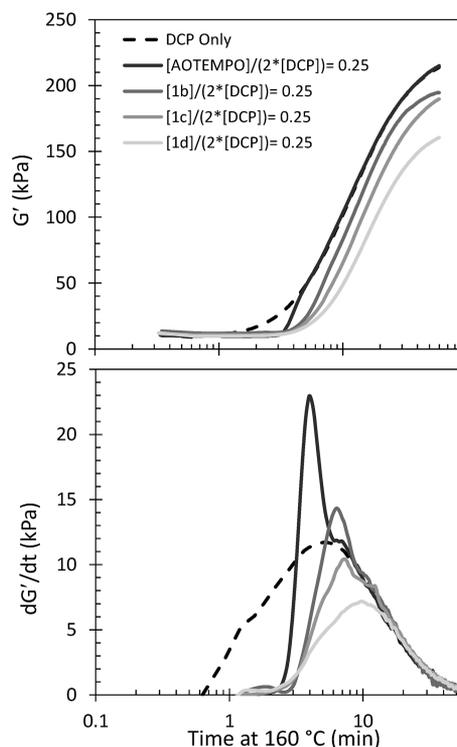
**Figure 7.** Storage modulus DCP-initiated LLDPE cures containing various functionalized nitroxyls ( $[\text{DCP}] = 18.5 \mu\text{mol/g}$ ;  $[\text{nitroxyl}] = 9.3 \mu\text{mol/g}$ ).
