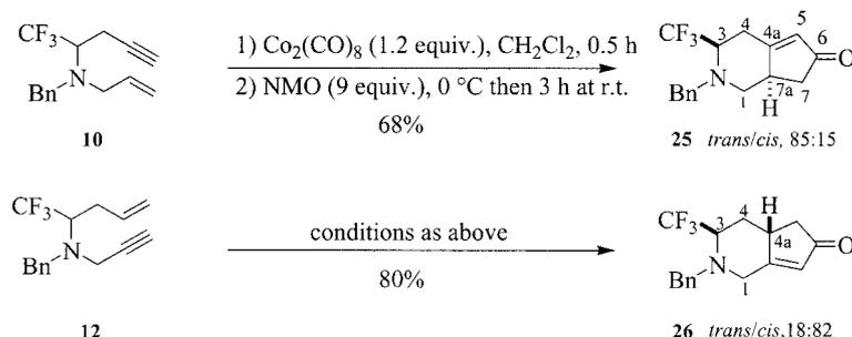
Scheme 2. Syntheses of CF<sub>3</sub>-containing heterobicyclic compounds **25** and **26** by a Pauson–Khand reaction.
