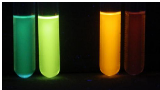
Fig. 7. Photoluminescence of C2 and C6 in the solvents excited by 365 nm. From left to right: C2 , C6 in THF; C2 , C6 in acetonitrile.
