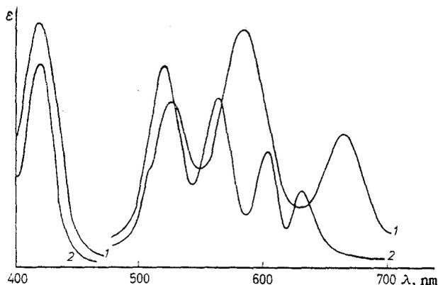
Fig. 1. Electronic absorption spectra of porphyrins in 5% KOH solution: 1) I and 2) II.
