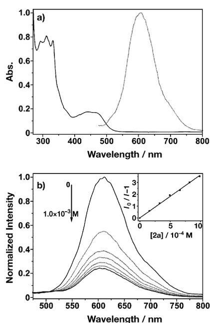
Figure 2. a) UV/Vis absorption and luminescence spectra of platinum(II) complex **1** ( $1.0 \times 10^{-5}$  M) in DMF. b) Luminescence spectra of platinum(II) complex **1** ( $1.0 \times 10^{-5}$  M) as a function of concentration of **2a** in degassed DMF with excitation at 450 nm. Inset is the Stern–Volmer plot of complex **1** by **2a**.
