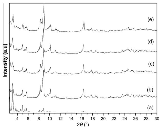
**Fig. 1.** Powder X-ray diffraction patterns of samples: (a) MIL-101(Cr), simulated; (b) MIL-101(Cr), activated; (c) MIL-101(Cr)-NH<sub>2</sub>; (d) Pd/MIL-101(Cr)-NH<sub>2</sub>, before reaction; (e) Pd/MIL-101(Cr)-NH<sub>2</sub>, after five runs of catalysis.
