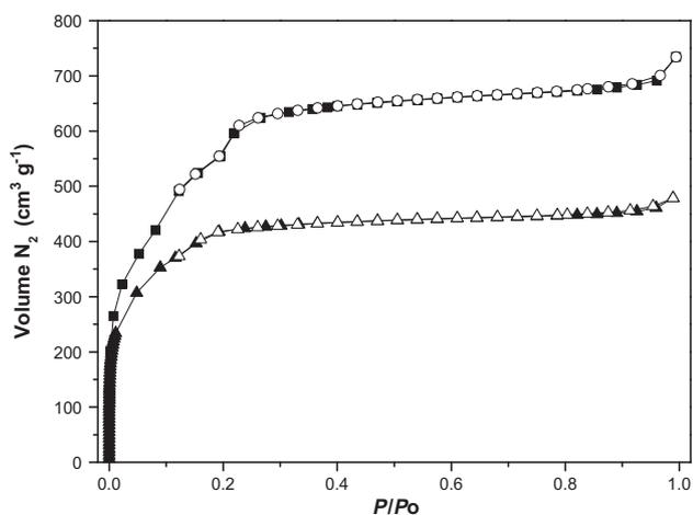
**Fig. 2.** Nitrogen sorption isotherms at 77.3 K for MIL-101(Cr)-NH<sub>2</sub> (■ = adsorption, □ = desorption) and Pd/MIL-101(Cr)-NH<sub>2</sub> (▲ = adsorption, △ = desorption).
