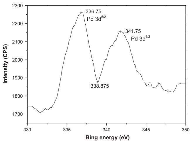
**Fig. 4.** XPS spectrum of a Pd/MIL-101(Cr)-NH<sub>2</sub> sample.
