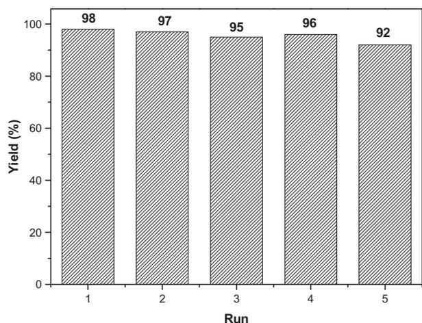
**Fig. 5.** Recycling of Pd/MIL-101(Cr)-NH<sub>2</sub> for five runs of the dehalogenation of 4-chlorophenol at room temperature for 3 h.
