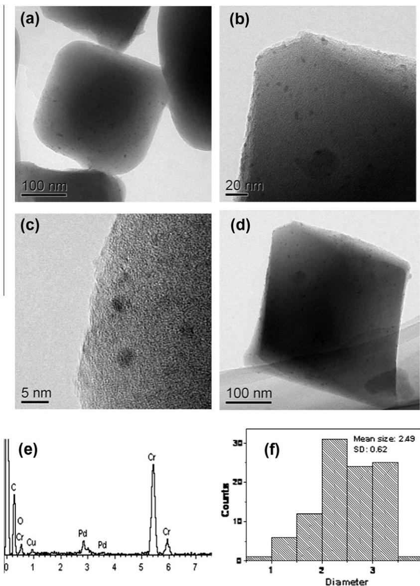
**Fig. 3.** Transmission electron microscopy (a and b) and high-resolution transmission electron microscopy (c) images of Pd/MIL-101(Cr)-NH<sub>2</sub> (0.62 wt% Pd) before the reaction and after five catalytic cycles (d), the energy-dispersive X-ray spectroscopy (EDS) pattern (e), and the size distribution of Pd NPs (f).
