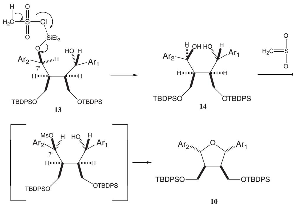
**Scheme 4.** Proposed Mechanism for the Production of Diol **14** and Tetrahydrofuran Derivative **10** from Benzyl Alcohol **13**. Ar<sub>1</sub>, 3,4-methylenedioxyphenyl; Ar<sub>2</sub>, 3,4-dimethoxyphenyl
