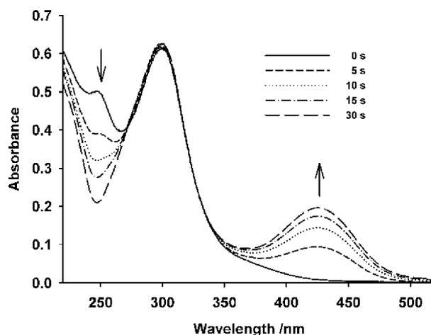
**Figure 1.** UV–Vis absorption spectra for an aqueous solution of **19** upon 300-nm irradiation for the cumulative time periods indicated. The arrows indicate the direction of absorbance changes with increasing irradiation time.
