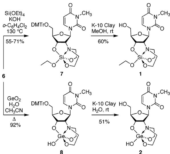
silicate provided 55–71% yield of silatrane **7**, Scheme 2. Alternatively, **6** was heated with germanium dioxide<sup>23</sup> in acetonitrile–water to provide 92% yield of germatrane **8**. Detritylation of **7** and **8** was best accomplished by treatment with montmorillonite K 10 (K-10 clay)<sup>24</sup> to produce silatranyluridine **1** and germatranyluridine **2** in 60 and 51% yields, respectively.
