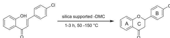
Scheme 1. Isomerisation of 2'-hydroxychalcones to flavanone using silica supported DMC.
