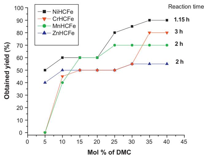
Fig. 6. Effects of mol% of DMCs on yields at 100 °C for Zn-, Ni-, Mn-HCFE and 150 °C for CrHCFE.
