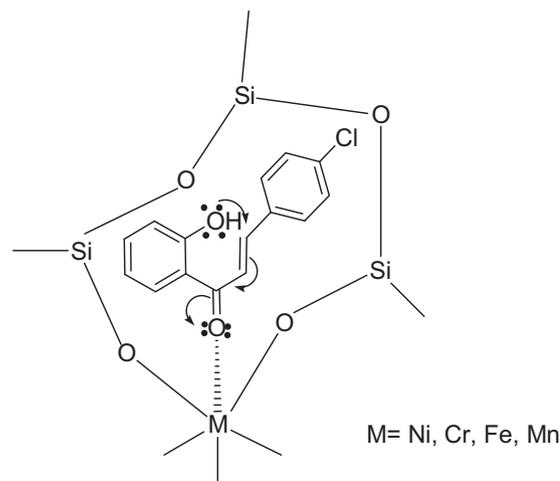
**Scheme 2.** Proposed mechanism for isomerisation of 2'-hydroxychalcones using silica supported DMCs catalysts.
