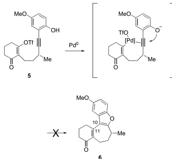
Scheme 2. Initial strategy for the key cyclization in the synthesis of frondosin B (**1**). Tf = trifluoromethanesulfonyl.
