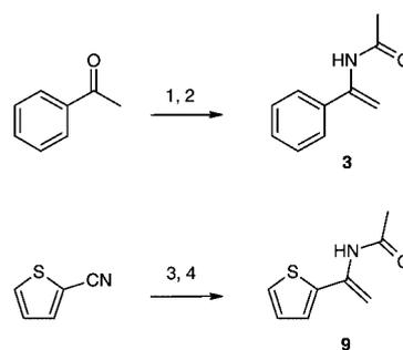
**Scheme 2.** Synthesis of substrates;<sup>[11,13,20,28]</sup> 1:  $\text{H}_2\text{NOH HCl}$ , EtOH, pyridine; 2:  $\text{Ac}_2\text{O}$ , AcOH, Fe, TMSCl, toluene; 3: MeMgBr,  $\text{Et}_2\text{O}$ ; 4:  $\text{Ac}_2\text{O}$ ,  $\text{Et}_2\text{O}$ .
