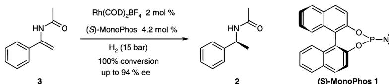
**Scheme 1.** Hydrogenation using monodentate phosphoramidite MonoPhos **1**.
