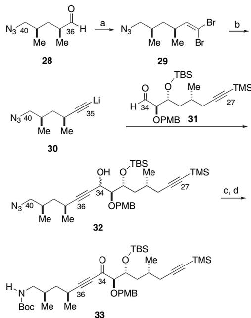
**Scheme 6.** Assembly of the DIHMA precursor. a)  $\text{CBr}_4$ ,  $\text{Ph}_3\text{P}$ ,  $\text{CH}_2\text{Cl}_2$  (91%); b) *n*-BuLi, THF,  $-78^\circ\text{C}$ , then **31** (70%); c) (i)  $\text{Et}_3\text{P}$ , toluene, (ii) BocON,  $-10^\circ\text{C}$  to rt (61%); d)  $\text{MnO}_2$ , pentane (100%).
