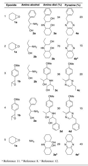
In conclusion, we have developed what appears to be a versatile route to symmetrical and unsymmetrical pyrazines. It is particularly noteworthy that the Swern oxidation of the aminodiols can be carried out without protection of the basic amines.
