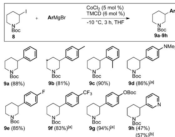
**Scheme 7.** Cross-coupling involving 3-iodopiperidine **8**. [a] Grignard reagent prepared as  $\text{ArMgBr}\cdot\text{LiCl}$ .<sup>[29]</sup> [b] Using 50 mol% of TMCD.
