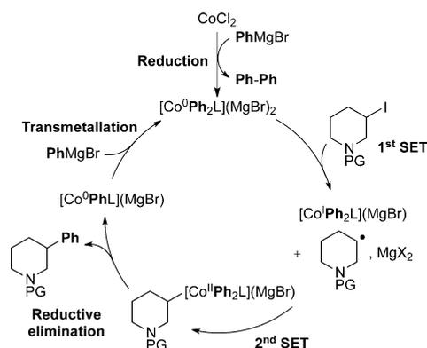
Scheme 9. Hypothetical mechanism for the Co-catalyzed cross-coupling. SET: single-electron transfer.
