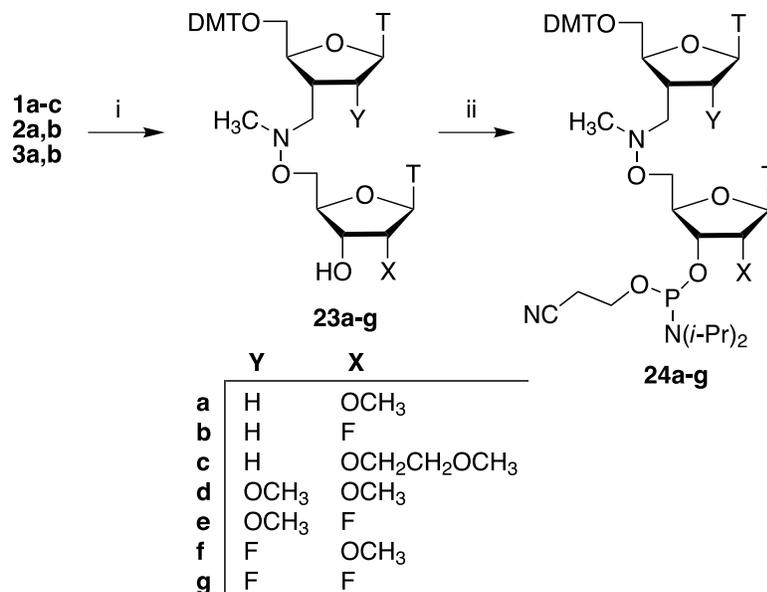
**Scheme 6.** Reagents and Conditions: (i) DMTCl/pyridine/DMAP; (ii) 2-cyanoethyl-*N,N,N',N'*-tetraisopropylphosphorodiamidite/diisopropylammonium tetrazolide/CH<sub>2</sub>Cl<sub>2</sub> or 2-cyanoethyl-*N,N*-diisopropylchlorophosphoramidite/*(i-Pr)*<sub>2</sub>NEt/THF.
