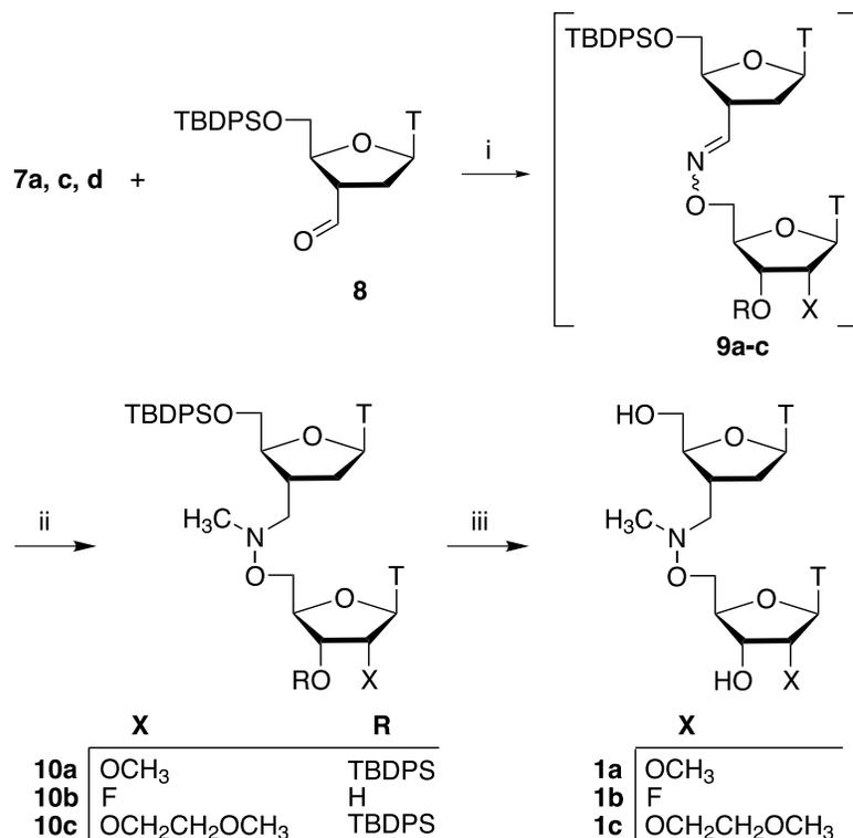
**Scheme 2.** Reagents and Conditions: (i) PhCH<sub>3</sub>/CH<sub>2</sub>Cl<sub>2</sub>/catalytic AcOH; (ii) NaBH<sub>3</sub>CN/CH<sub>2</sub>O/AcOH; (iii) TBAF/THF.
