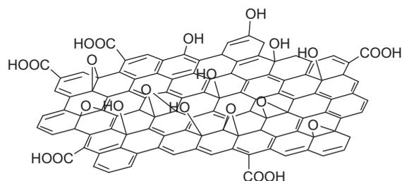
Figure 1. Schematic representation of graphene oxide.
