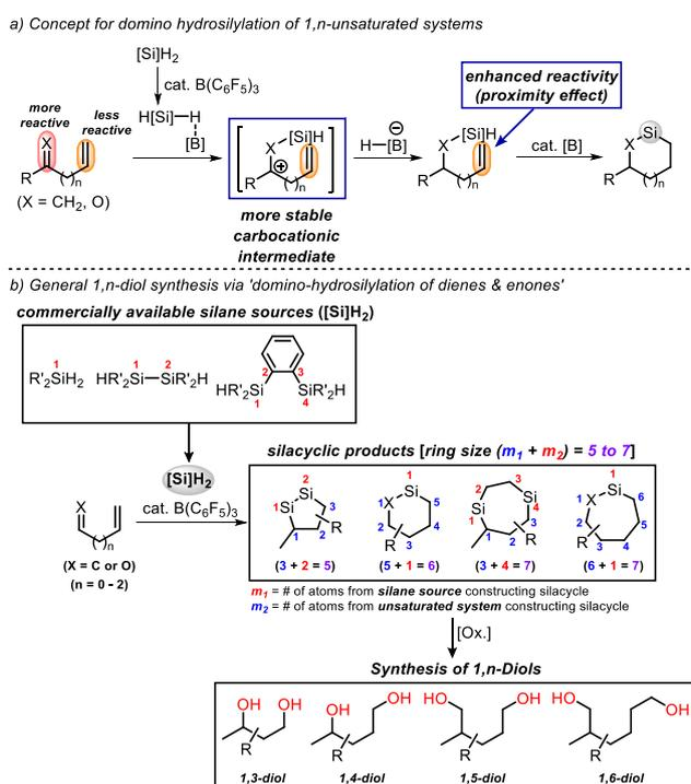
**Scheme 1.** Synthesis of 1, $n$ -diols via [B(C<sub>6</sub>F<sub>5</sub>)<sub>3</sub>]-catalyzed domino hydrosilylation
