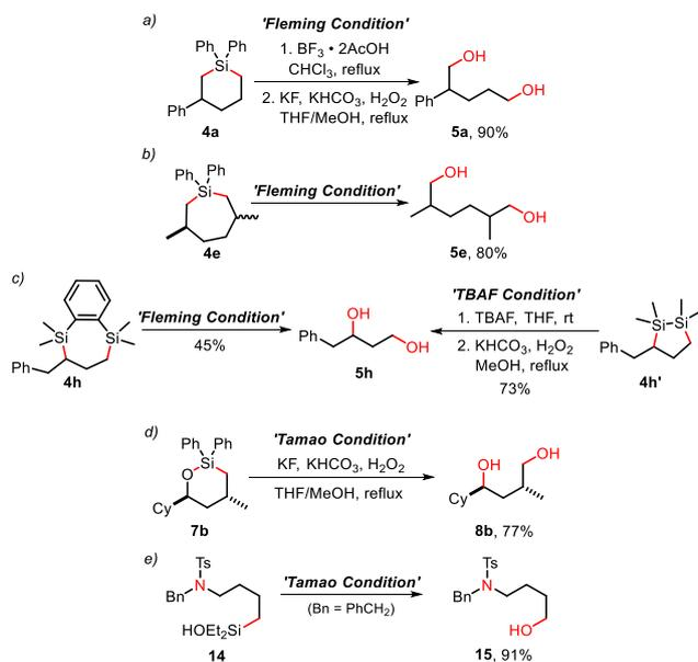
**Scheme 5.** Conversion of silacycles to the corresponding diols via oxidation
