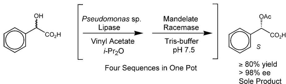
**Scheme 4.** Deracemization of ( $\pm$ )-mandelate using a stepwise two-enzyme process.
