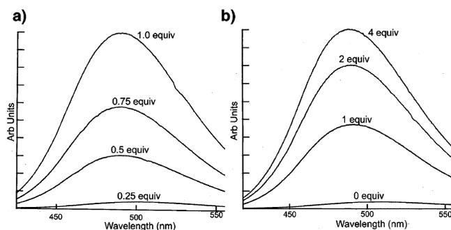
**Figure 2.** (a) Emission fluorescence spectra of  $10^{-5}$  trinsyl **2** in  $\text{CH}_3\text{CN}$ , titrated with  $\text{CF}_3\text{CO}_2\text{H}$ : 0, 0.25, 0.50, and 1 equiv. (b) Emission fluorescence spectra of  $10^{-5}$  trinsyl **2** in  $\text{CH}_3\text{CN}$ , titrated with  $\text{ZnCl}_2$ : 0, 1, 2, and 4 equiv ( $\lambda_{\text{ex}} = 332$  nm).
