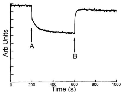
**Figure 5.** Plot of fluorescence emission intensity ( $\lambda_{em} = 472$  nm;  $\lambda_{ex} = 332$  nm) vs time for a stirred suspension of macroporous cross-linked poly(ethylene glycol)dimethacrylate doped with probe **5** in CH<sub>2</sub>Cl<sub>2</sub>. Time A (arrow) corresponds to addition of diethylamine (4:1 amine:probe) and time B (arrow) corresponds to addition of CF<sub>3</sub>CO<sub>2</sub>H (4:1 acid:probe).
