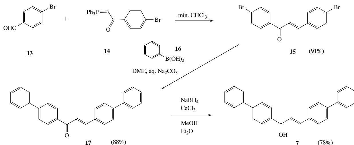
**Scheme 7.** Preparation of 1,3-bis(biphenyl)prop-2-en-1-one (17) and 1,3-bis(4-biphenyl)-prop-2-en-1-ol (7).
