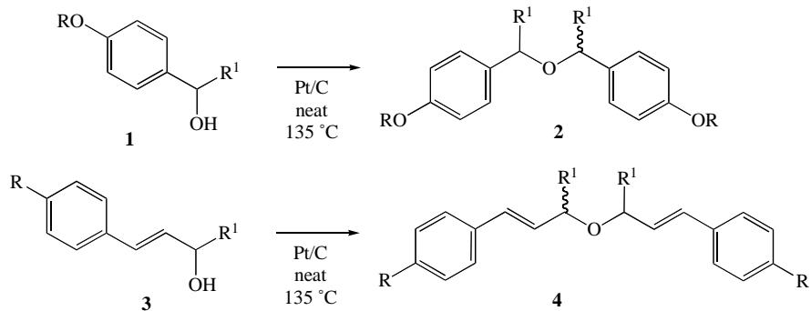
**Scheme 1.** Etherification of 4-alkoxyphenyl alkyl carbinols and cinnamyl alkyl carbinols in the presence of Pt/C [8].
