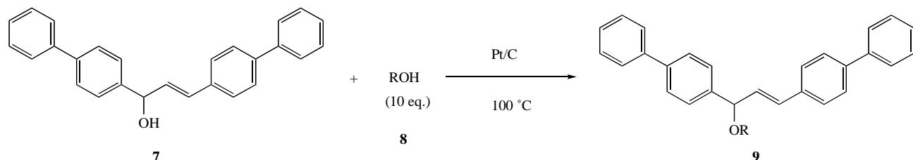
**Scheme 3.** Etherification of 1,3-bis(4-biphenyl)-prop-2-en-1-ol over Pt/C.
