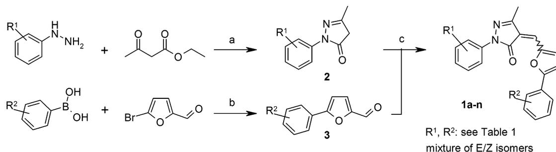
**Scheme 3.** Reagents and conditions: (a) acetic acid, reflux, 3 h; (b) Pd(PPh<sub>3</sub>)<sub>4</sub>, Na<sub>2</sub>CO<sub>3</sub> aqueous 2 M, toluene, methanol, reflux, 3 h; or Pd(PPh<sub>3</sub>)<sub>4</sub>, CsF, toluene, methanol, 60 °C, overnight; (c) acetic acid, sodium acetate, reflux, 3 h.
