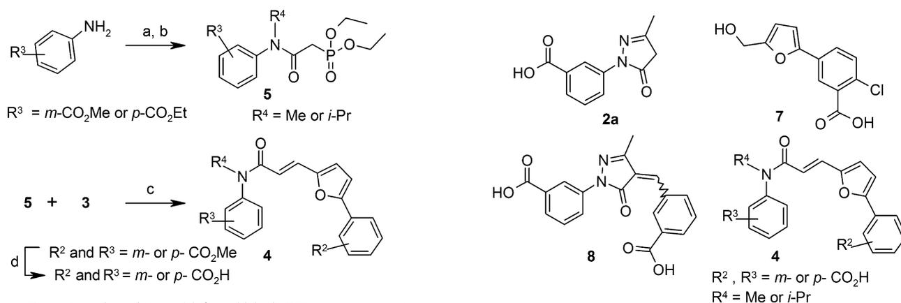
**Scheme 4.** Reagents and conditions: (a) formaldehyde 37% aqueous or acetone, NaBH<sub>3</sub>CN 1 M in THF, acetic acid, THF, rt, overnight; (b) (diethoxy)phosphorylacetic acid, 2-chloro-1-methyl-pyridinium iodide, TEA, dichloromethane, rt, overnight; (c) LiCl, DIPEA, acetonitrile, rt, overnight; (d) LiOH, THF, water, rt, overnight.
