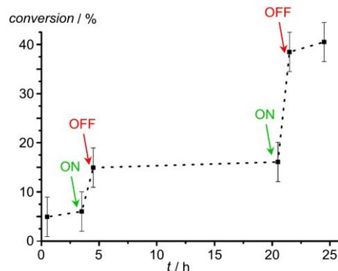
**Fig. 3** Conversion versus time plot of the cyclisation (Scheme 1) during ON/OFF redox switching using Magic Blue (1.00/1.05 eq; ON) and FeCp\*<sub>2</sub> (1.05/1.10 eq; OFF).
