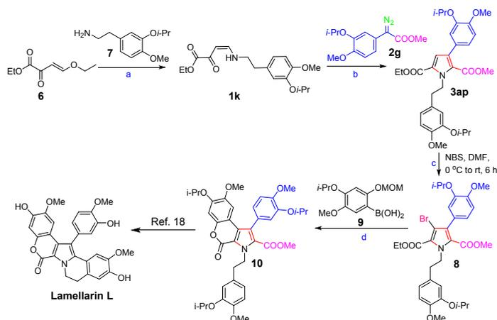
Reaction conditions: <sup>a</sup>Stirred in THF for 12 h at 20–60 °C, 87%. <sup>b</sup>Cat. AgOTf (5 mol%), CH<sub>2</sub>Cl<sub>2</sub>, stirred for 12 h at rt, 68%. <sup>c</sup>NBS, DMF, 0 °C to rt, 6 h, 99%. <sup>d</sup>**9** (2.0 equiv.), Pd(PPh<sub>3</sub>)<sub>4</sub> (10 mol%), THF, reflux, 18 h, 2) concd HCl, MeOH, reflux 1 h (two-step, 94%).
