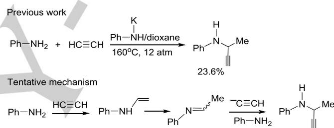
**Scheme 1.** Superbase-catalyzed one-pot synthesis of 3-arylamino-1-butyne from aniline and acetylene.<sup>[12]</sup>
