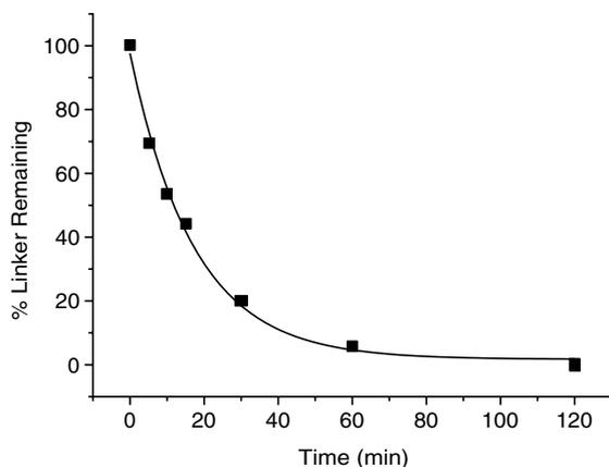
**Figure 2.** Rate of photolysis of **6** by exposure to UV light ( $\lambda_{\text{max}} = 365$  nm) from a pyrex-filtered 16 W mercury vapour fluorescent lamp was determined by integrating the NMR signal corresponding to H3 ( $\delta$  7.90).
