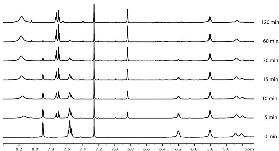
**Figure 1.** Photolysis of **6** by exposure to UV light ( $\lambda_{\text{max}} = 365$  nm) from a pyrex-filtered 16 W mercury vapour fluorescent lamp, as followed by  $^1\text{H}$  NMR.
