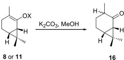
**Scheme 4.** Conditions: From **8** (X=COCH<sub>3</sub>): 15 min, rt (*cis/trans*: 1/3; 66%). From **11** (X=COC<sub>6</sub>H<sub>5</sub>): 24 h, rt (*only trans*; 50%).
