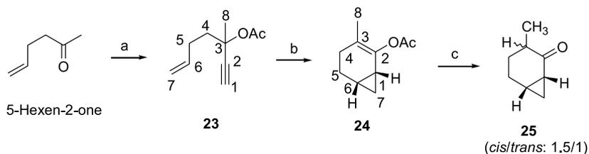
**Scheme 7.** Reagents: (a) Ethynylmagnesium bromide, THF/Et<sub>2</sub>O (1:1), rt, 3 h (50%); then, Ac<sub>2</sub>O, py, DMAP, rt, 12 h (67%); (b) PtCl<sub>2</sub> (5%), toluene, rt, 18 h (99%); (c) K<sub>2</sub>CO<sub>3</sub>, MeOH, rt, 18 h (61%).
