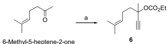
**Scheme 3.** Reagents: (a) Ethynylmagnesium bromide, 2 h, rt; then  $\text{ClCO}_2\text{Et}$ , py, DMAP, 5 h, rt (68%).
