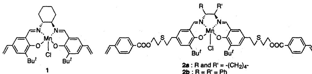
Enantiopure Mn(III)-salen complexes **1**, **2a** and **2b** (Figure 1), all of them bearing styrene-type vinyl groups, were submitted to radical copolymerization with styrene and divinylbenzene in the presence of AIBN (Figure 2). The reaction was carried out in oxygen-free toluene at 100°C, and the monomeric ratio in the reaction mixture was 10:75:15 for the Mn-salen, styrene, and divinylbenzene, respectively.<sup>9</sup>
