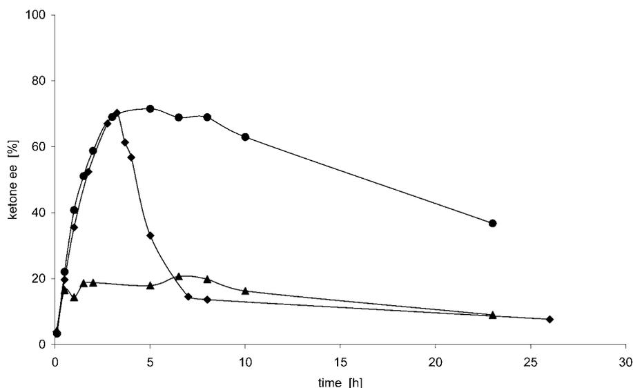
**Figure 4.** Analytical scale DKR of *rac*-1. Effect of Lewatit MP62 on unreacted ketone ees. No resin: ●; addition of resin (24.5 meq L<sup>-1</sup>) at time 0: ▲; after 3.5 h: ◆ (other conditions: 1 g L<sup>-1</sup> of *rac*-1, pH 7.5, 30 °C).
