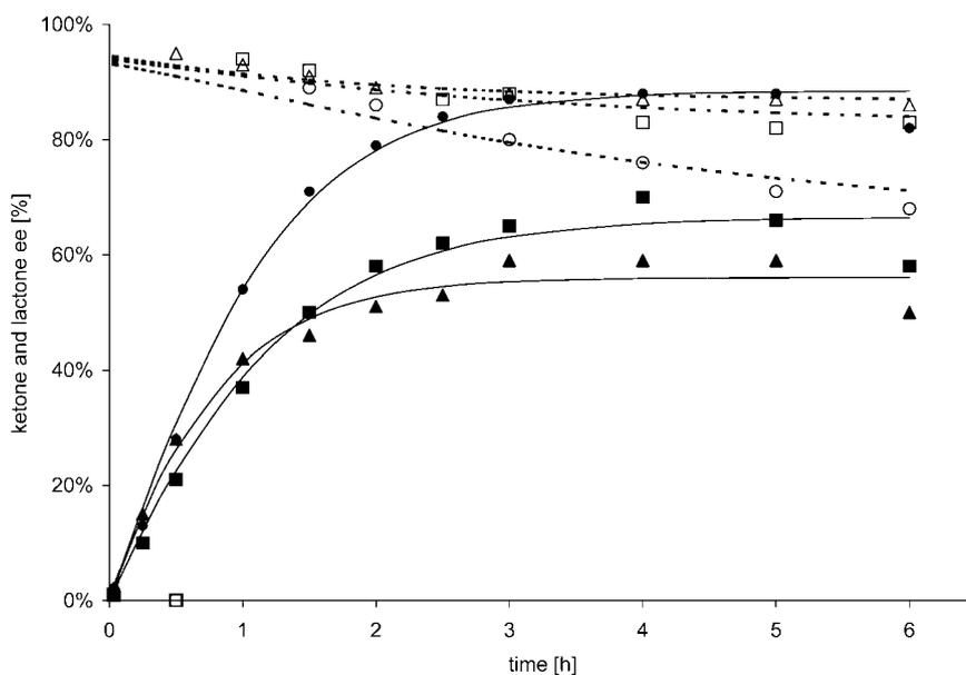
**Figure 5.** Analytical scale DKR of *rac*-1: Experimental and simulated effect of Lewatit MP62 on ketone and lactone ees. Experimental (symbol) and simulated (line) ketone (empty symbol) and lactone (black symbol) ees. No resin: ○ and ●; Lewatit MP62 4 meq L<sup>-1</sup>: □ and ■; 8 meq L<sup>-1</sup>: △ and ▲ (others conditions: 0.3 g L<sup>-1</sup> of **1**, pH 7.5, 37 °C).
