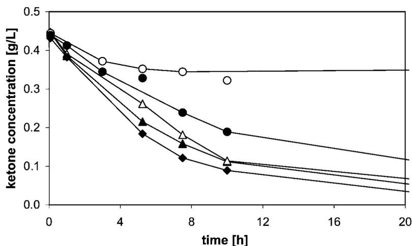
**Figure 3.** Determination of the inhibitory level of lactone **2**. Time dependent concentration of *rac*-**1** in the presence of various initial concentrations of *rac*-**2**: ◆ 0, ▲ 0.5, △ 0.7, ● 1.0 and ○  $1.5 \text{ g L}^{-1}$  (other conditions:  $30^\circ\text{C}$ , pH 7,  $0.5 \text{ g L}^{-1}$  of *rac*-**1**).
