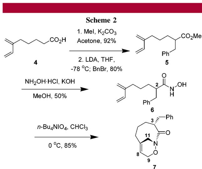
of 6-methylene-7-octenoic acid **4**<sup>8</sup> followed by alkylation (LDA, THF,  $-78$  °C; BnBr) provided ester **5**. Conversion of **5** to hydroxamic acid **6** was accomplished by treatment with  $\text{NH}_2\text{OH}\cdot\text{HCl}$  and KOH in MeOH. Addition of hydroxamic acid **6** to a  $\text{CHCl}_3$  solution of *n*- $\text{Bu}_4\text{NIO}_4$  led to the isolation of cycloadduct **7** in 85% yield as a *single diastereomer* (100% ds).<sup>17</sup>
