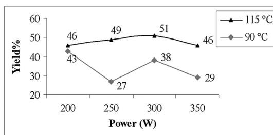
**Figure 2.** Microwave-assisted Hantzsch cyclization at different applied temperatures (°C) and powers (W).
