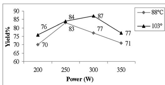
**Figure 1.** Microwave-assisted synthesis of 1-(propan-2-yliden)thiosemicarbazide in different conditions of applied temperature (°C) and power (W).
