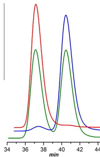
Figure 2. HPLC chromatograms of 3-(4-nitrophenoxy)propane-1,2-diol **1c**. Green curve: *rac*-**1c**; blue curve: **1c** diol obtained by using AD-mix- $\beta$ ; red curve: (*R*)-**1c**.
