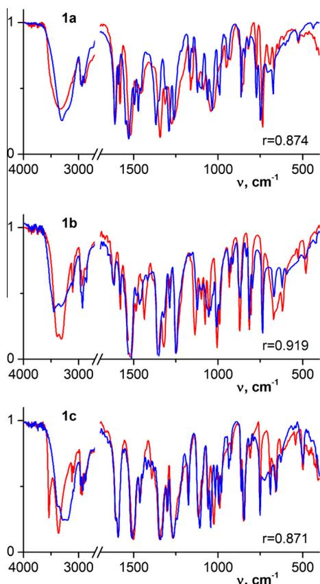
**Figure 4.** IR spectra of samples of racemic (red curves) and enantiopure (blue curves) **1a–c** and coefficients of correlation between them.
