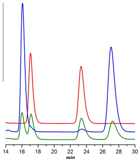
**Figure 3.** HPLC chromatograms of cyclic sulfites obtained on the basis of 3-(3-nitrophenoxy)-propane-1,2-diols **1b** (see Scheme 3). Green curves: *rac*-**1b** was used as the starting material; blue curves: diol **1b**, obtained by using AD-mix- $\beta$ , was used as the starting material; red curves: sulfites from (*R*)-**1b**.
