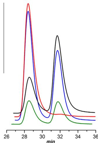
Figure 1. HPLC chromatograms of 3-(2-nitrophenoxy)propane-1,2-diol **1a**. Green curve—*rac*-**1a**; blue curve—diol **1a** obtained by dihydroxylation of nitrophenyl allyl ether **3a** using AD-mix- $\beta$ ; red curve—(*R*)-**1a**; black curve—(*R*)-**1a** obtained by dihydroxylation of nitrophenyl allyl ether **3a** using AD-mix- $\alpha$ .
