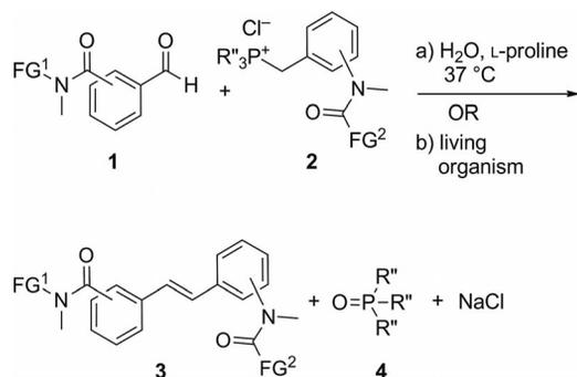
Scheme 1. Organocatalytic and bioorthogonal Wittig process. Synthesis of donor–acceptor flanked reporter stilbene **3** under mild chemical conditions and under physiological conditions.
