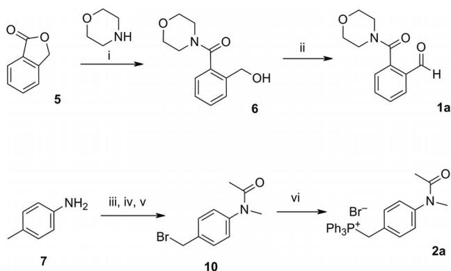
Scheme 2. Synthesis of aldehyde **1a** and phosphonium salt **2a**. Reagents and conditions: (i) morpholine, AlCl<sub>3</sub>, 1,2-DCE, r.t., 88%; (ii) (COCl)<sub>2</sub>, DMSO, Et<sub>3</sub>N, DCM, −78 °C, 84%; (iii) Ac<sub>2</sub>O, Et<sub>3</sub>N, DCM, r.t. gave **8** (99%); (iv) LiHMDS, MeI, THF, r.t. gave **9** (95%); (v) NBS, BPO, PhH, reflux, 3 h, (80%); (vi) PPh<sub>3</sub>, PhMe, reflux, 6 h, (96%).
