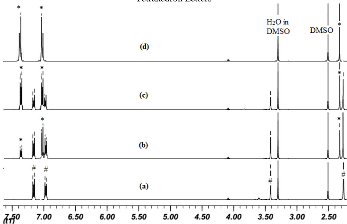
**Figure 1.** The  $^1\text{H}$  NMR (300 MHz) spectroscopic monitoring of conversion of **1b** to **2b** at ambient conditions: (a) at beginning of the reaction, (b) after 3 h, (c) after 6 h and (d) after 8 h. Notice that new peaks (\*) corresponding to **2b** gradually appeared at 2.31, 7.08 and 7.37 ppm, while signals (#) of **1b** at 2.28, 3.41, 7.01 and 7.16 ppm have been disappeared indicating the product formation.
