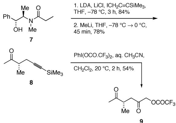
**Scheme 3.** Synthesis of Alcohol **5** (R = H) in Latent Form
