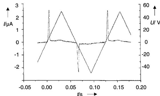
Figure 4. Switching current response in the mesophase of compound **4** on applying a triangular-wave voltage at  $104^\circ\text{C}$  in a  $10\ \mu\text{m}$  non-coated ITO cell (EHC, Japan) at a frequency of 1 Hz.
