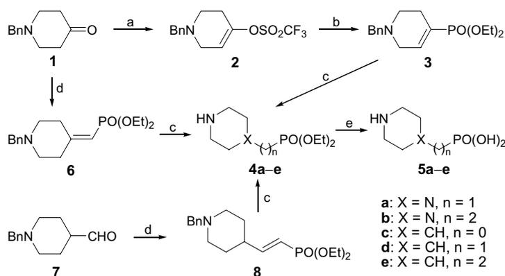
**Scheme 1.** (a) LDA, DME; then  $\text{PhN}(\text{SO}_2\text{CF}_3)_2$ ; (b) diethyl phosphite, cat.  $\text{Pd}(\text{PPh}_3)_4$ , DMF; (c)  $\text{Pd}/\text{C}$ ,  $\text{H}_2$  (1 atm), MeOH, rt; (d)  $\text{CH}_2[\text{PO}(\text{OEt})_2]_2$ , NaH, toluene; (e) 4 N aqueous HCl, reflux.
