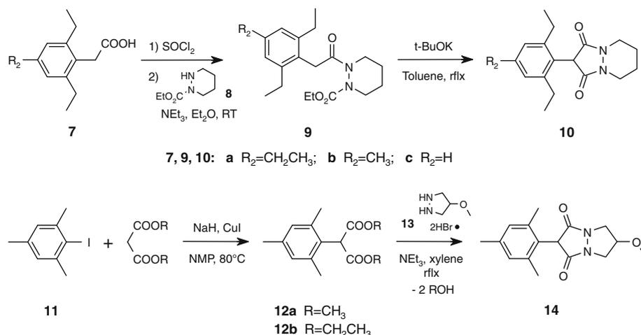
**Scheme 1.** General access to 4-aryl-pyrazolidine-3,5-diones via either a cyclization sequence (**10**) or a condensation route (**14**).
