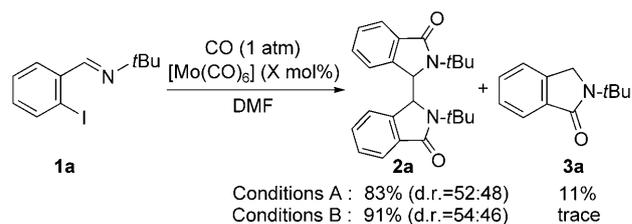
**Scheme 2.** Formation of bis(isoindolinone) **2a** by the carbonylative cyclization of **1a** with [Mo(CO)<sub>6</sub>] in the presence of the proton sponge. Conditions A: X = 100, 100 °C, 1.5 h. Conditions B: X = 30, proton sponge (200 mol%), 120 °C, 10 h. DMF = *N,N*-dimethylformamide.
