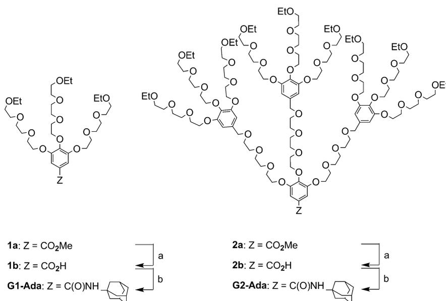
Scheme 1. Synthesis procedures for OEG-based dendritic guests **G1-Ada** and **G2-Ada**. Reagents and conditions: a) **1a** or **2a**, LiOH·H<sub>2</sub>O, MeOH/H<sub>2</sub>O, -5 to 25 °C, 12 h, (97% and 75% for **1b** and **2b**, respectively); b) **1b** or **2b**, 1-adamantaneamine, EDC, HOBt, TEA, DCM, -15–25 °C, overnight (56% and 71% for **G1-Ada** and **G2-Ada**, respectively).<sup>[39]</sup>
