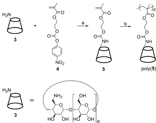
Scheme 2. Synthesis procedures for the host polymer poly(5). Reagents and conditions: a) **3**, **4**, DiPEA, DMF/MeOH, -15–25 °C, overnight, 53%; b) **5**, AIBN, DMF, 60 °C, 12 h, 40%.
