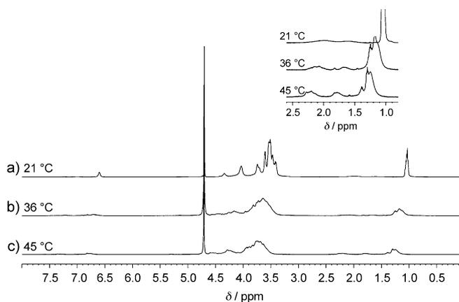
Figure 6. Temperature-dependent  $^1\text{H}$  NMR spectra of **SPG2**: a) 21 °C, b) 36 °C, c) 45 °C. The inset shows partial spectrum in the range of  $\delta = 1.0\text{--}2.5$  ppm.
