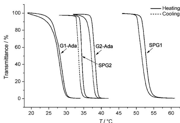
Figure 4. Plots of transmittance versus temperature for 0.25 wt % aqueous solution **G1-Ada**, **G2-Ada**, **SPG1**, and **SPG2**.
