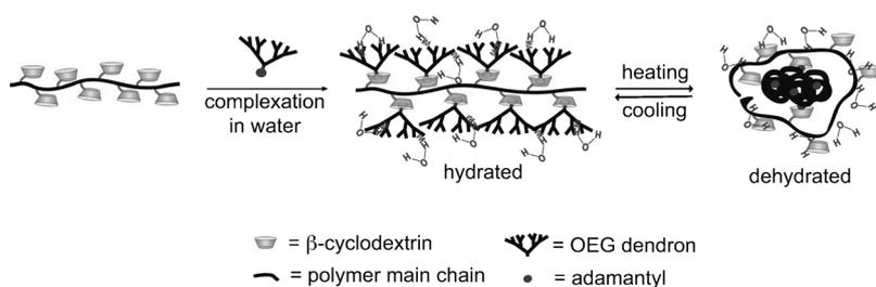
Figure 1. Illustration of side-chain supramolecular dendronized polymers (SDPs) prepared through host-guest inclusion and their collapse in water.
