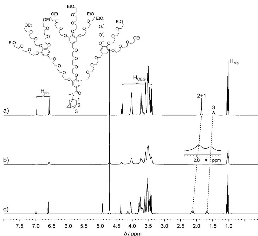
Figure 2. <sup>1</sup>H NMR spectra at room temperature in D<sub>2</sub>O (with the same **G2-Ada** concentration at 1.6 × 10<sup>-2</sup> mol L<sup>-1</sup>) of a) pure **G2-Ada**, b) the mixture of 1 equivalent of **G2-Ada** and poly(5), and c) the mixture of 1 equivalent of **G2-Ada** and β-CD. The dotted lines are a guide for the eyes.
