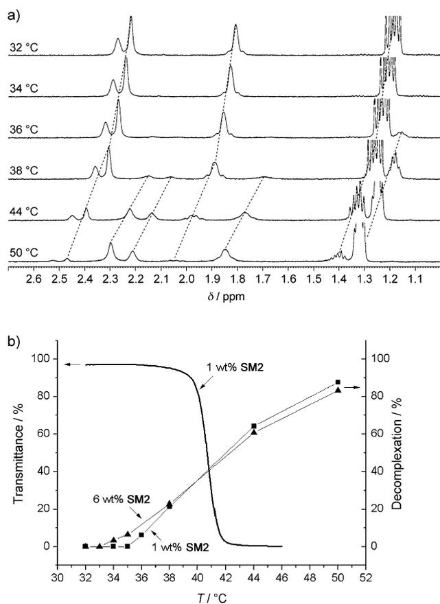
Figure 7. a) Temperature-dependent <sup>1</sup>H NMR spectra of 1 wt % aqueous solution of **SM2**. The dotted lines are a guide for the eyes. b) Plots of transmittance and dissociation percentage versus temperature for 1 wt % and 6 wt % aqueous solutions of **SM2** (the solid lines between the plots are a guide for the eyes).
