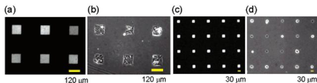
**Figure 3.** Cell attachment to array-patterned spots corresponding to photomasks inserted at the location of the field diaphragm of a fluorescence microscope. (a and c) Fluorescence images of glass coverslips painted with a fluorescent pen, which were irradiated using corresponding photomasks. (b and d) Phase-contrast images of HEK293 and COS7 attached on the substrates 18 and 2.5 h after seeding, respectively.
