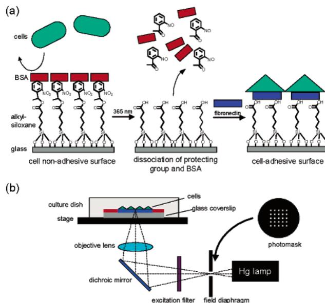
**Figure 1.** Schematic representations of photoactivation of cell adhesion. (a) UV-directed replacement of BSA with fibronectin changed the surface from a state that prevents cell adhesion to a state that promotes cell adhesion. (b) Experimental setup for irradiation under a standard fluorescence microscope.
