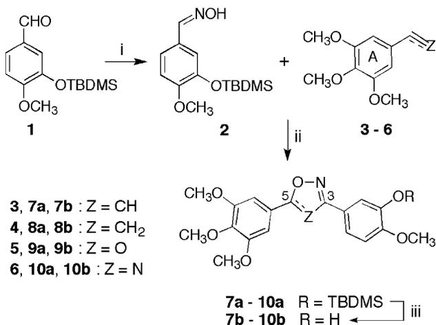
Scheme 1. Reagents and conditions: (i) NH<sub>2</sub>OH·HCl, pyridine, EtOH, reflux, 1 h; (ii) aq NaOCl, Et<sub>3</sub>N, CH<sub>2</sub>Cl<sub>2</sub>, 0 °C, then rt 24 h (additional reflux 24 h for **5** and **6**); (iii) TBAF, THF, rt, 2 h.
