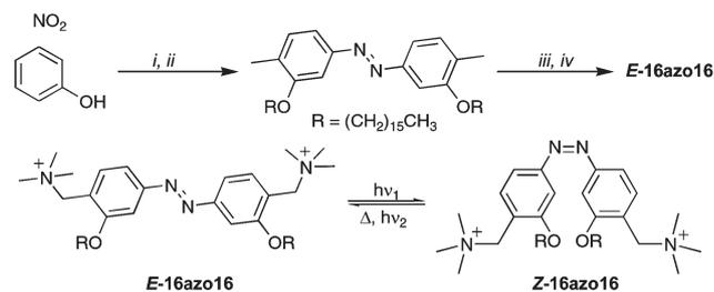
**Scheme 1** Synthesis and photoisomerisation of 16azo16. *i*, RI, K<sub>2</sub>CO<sub>3</sub>, 18-crown-6, THF, 80 °C (95%); *ii*, LiAlH<sub>4</sub>, THF, 80 °C (30%); *iii*, NBS, CCl<sub>4</sub>, reflux (50%); *iv*, Me<sub>3</sub>N, CH<sub>3</sub>CN, 20 °C (90%).
