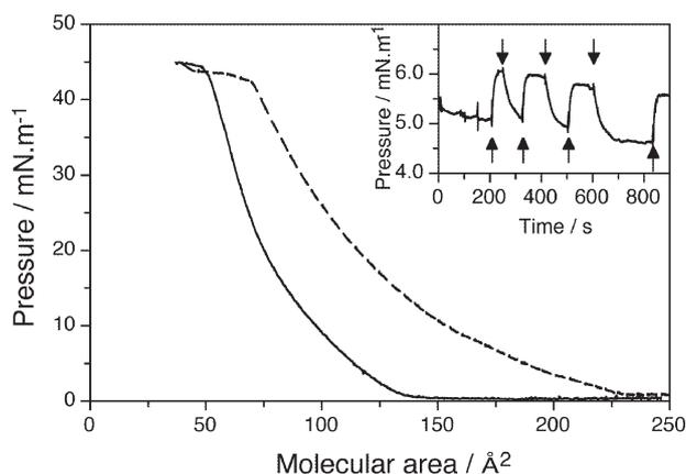
**Fig. 2** Effect of 365 nm irradiation on  $\pi$ -A isotherms of 16azo16 at the air–water interface. Solid line: *E*-16azo16. Dashed line: 1 : 1 mixture of *E*- and *Z*-16azo16 obtained by pre-irradiation of the sample prior to deposition. Inset shows the pressure response of the balance held at constant area (ca. 110 Å<sup>2</sup>/molecule) upon irradiation with a multiband UV-254/365 nm lamp (8W, up arrows: 365 nm, down arrows: 254 nm).
