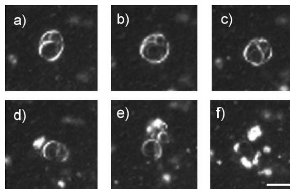
**Fig. 4** Rupturing of vesicles under irradiation. Images are taken every 10 s. Scale bar 15 μm.
