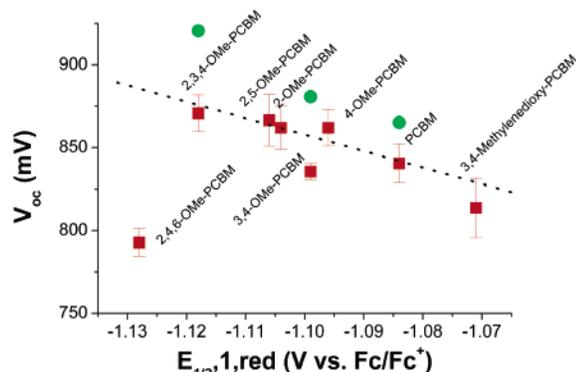
**Figure 2.**  $V_{oc}$  of devices from MDMO–PPV blends vs the first reduction potential,  $E_{1/2,1,red}$  (V vs ferrocene/ferrocene<sup>+</sup>) of the PCBM derivatives: squares, from ODCB; circles, from chlorobenzene. The dotted line is to guide the eye for a 1:1 relationship between  $V_{oc}$  and  $E_{1/2,1,red}$ .
