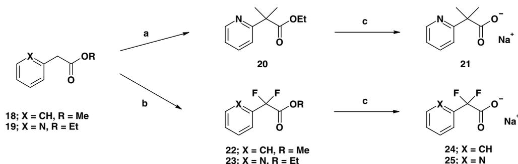
**Scheme 4.** Reagents and conditions: (a) THF, *t*-BuOK, rt, 10 min, then MeI, cooling (water bath), 1 h; (b) THF, potassium bis(trimethylsilyl)amide, -78 °C, 45 min, then  $\text{MnBr}_2$ , 30 min, then *N*-fluorobenzenesulfonamide, -78 °C for 30 min then warmed to rt the stirred 3 h; (c) 2 M  $\text{NaOH}$ , rt.
