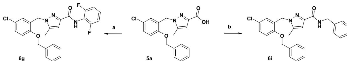
**Scheme 1.** Reagents and conditions: (a) i— $\text{CH}_2\text{Cl}_2$ ,  $(\text{COCl})_2$ , rt, 2 h, evaporation; ii— $\text{CH}_2\text{Cl}_2$ ,  $\text{NEt}_3$ , 2,6-difluoroaniline, rt, 2 h; (b)  $\text{BnNH}_2$ , HOBT, *N*-(3-dimethylaminopropyl)-*N'*-ethylcarbodiimide hydrochloride,  $\text{CH}_2\text{Cl}_2$ , rt.
