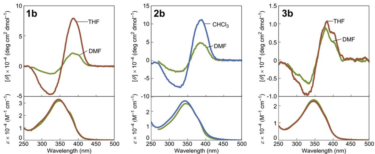
Fig. 3. CD and UV-vis spectra of **1b–3b** measured in  $\text{CHCl}_3$ , THF and DMF at room temperature ( $c = 0.03$  mM).
