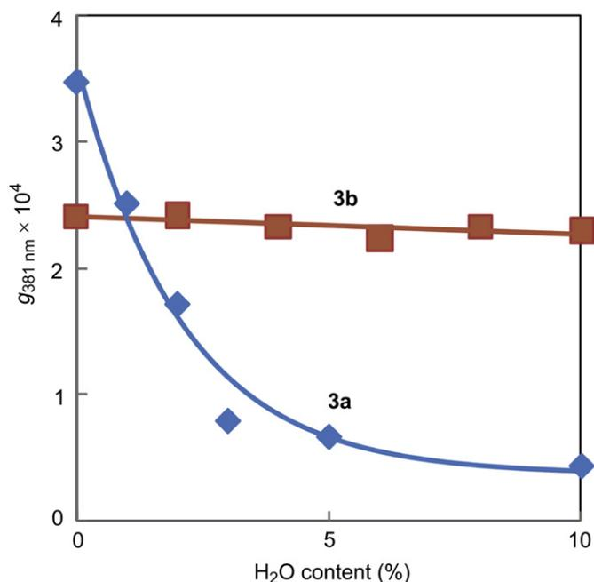
**Fig. 2.** Relationship between  $g$  values at 381 nm and  $\text{H}_2\text{O}$  content [ $\text{H}_2\text{O}/(\text{H}_2\text{O} + \text{THF})$ , volume ratio] of a solution of **3a** and **3b** in  $\text{THF}/\text{H}_2\text{O}$  ( $c = 0.03$  mM) at room temperature.
